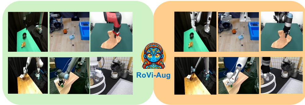
Figure 1: Given robot images, RoVi-Aug uses state-of-the-art diffusion models to augment the data and generate synthetic images with different robots and viewpoints. Policy trained on the augmented dataset can be deployed on the target robots zero-shot or further finetuned, exhibiting robustness to camera pose changes.
